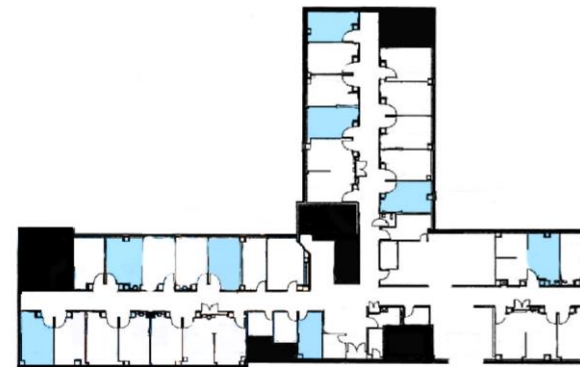
Beds designated for stroke care (light blue) are scattered throughout the ward. This is not ideal and does not align to the co-location component
